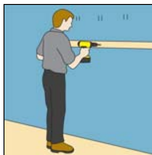
Fix a temporary timber
