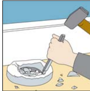
Remove the mortar around the collar of the waste pipe.
